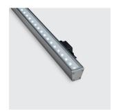
Linealuce compact - Wall-/Ceiling-mounted - 11Warm White LEDs 19W 965lm - 100-277V ac - L=528mm - Wall Washer Optic
